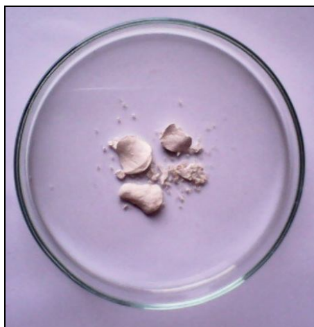
Fig. 8. Purified form of polyhydroxybutyrate (PHB) produced by CMBL-BT-6 strain of Bacillus thuringiensis under optimized culture conditions in nutrient broth (pH 7) containing 3.0% glucose as substrate, 0.1% ammonium sulphate as nitrogen source and 1% maltose as carbon source incubated at 37°C for 24 h.
